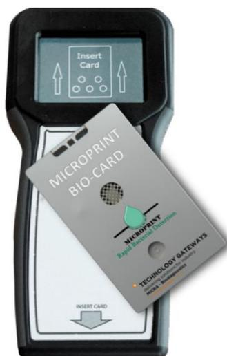
**MICROPRINT BIO-CARD & HANDHELD READER** is under development at MiCRA for the detection of bacteria in water and food samples. In water testing, a water sample is injected through a sampling strip which is then inserted into the BIO-CARD. After a period for on-cartridge culturing, the card is introduced to the handheld reader for processing. Readout follows in minutes identifying the micro-organism and cell count.
